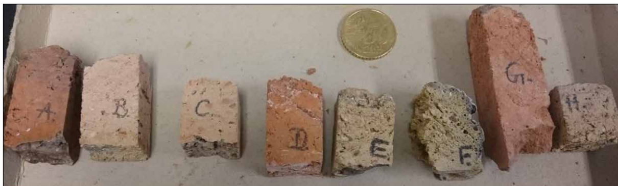
Figure 2 (above). Daub samples machined to \sim 20 \times 20 mm rectangular bars.
