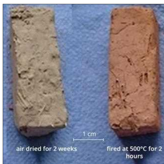
Figure 6. Daub bricks after air drying (left) and firing at 550°C (right).
