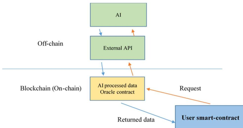
Figure 1: Traditional interaction of AI with smart contracts via an oracle
