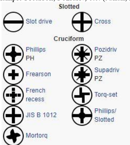
(Figure 2.4.2. Types of Slotted and Cruciform Screw drives, Linda Yen & Associates, Inc.)
